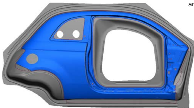
side panel Fiat 500, sheet metal after drawing
